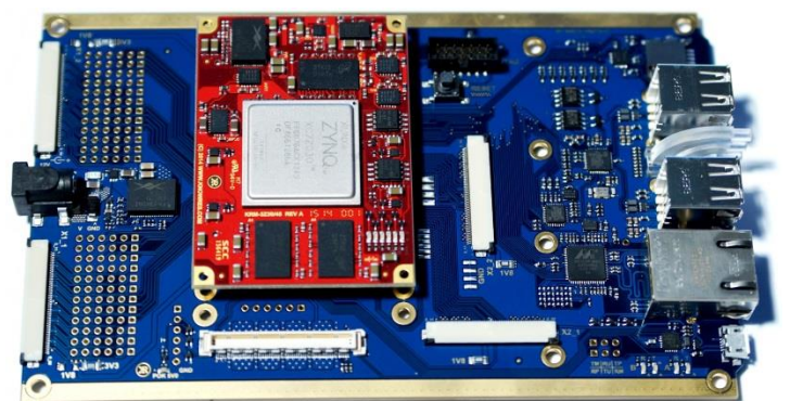
GbE, 4x USB, uSD, 2x UART to USB, 4 x exp port, MGT access, PMOD
