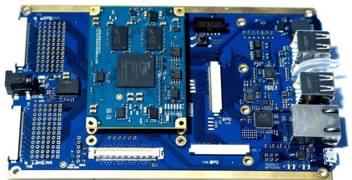
GbE, 4X USB, uSD, 2X UART to USB, 4 exp ports, PMOD support
